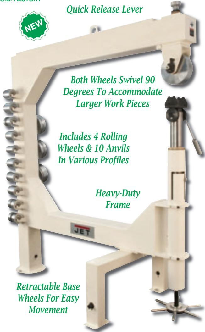
English wheel gets its name from the two steel wheels between which metal is formed. The wheels - one above and one below - are rolled against one another with a piece of sheet metal between, under a pre-adjusted pressure setting. The wheels roll as the sheet metal is moved back and forth. Shaping results as the lower wheel is forced under pressure into the metal, stretching and forming it.
